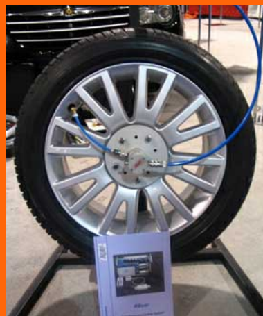
The new IPW Tire Pressure Monitoring system enables dynamic air pressure monitoring while the wheel is in motion.
