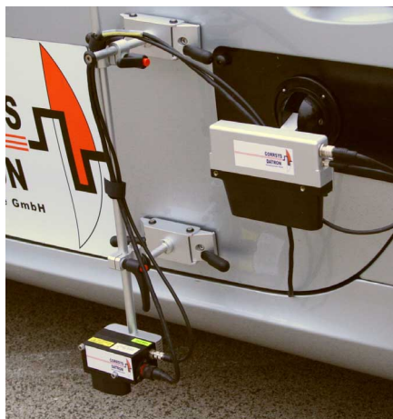
An HF-250 Sensor mounted alongside a CORREVIT® SF II-P Optical Sensor (bottom).
