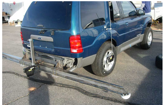
Instrumented for NHTSA fishhook testing, the SUV shown here is fitted with one CORREVIT® S-400 Optical Speed & Distance Sensor (rear), and four HT-500 Height Sensors.
