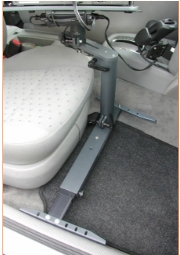
The bolt-on configuration is mounted using the bolts that secure the fronts of the seat rails.
