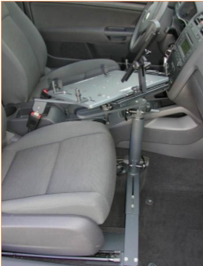
The spring-loaded configuration expands between the door sill board and the center tunnel to hold the unit firmly in place.
