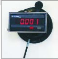
Compact Display for displaying velocity, etc. Analog input 0 ... 10 V conversion factor user selectable max. 20 scaling points sensor linearization
