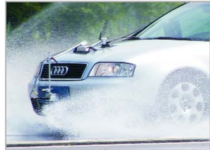
CORREVIT® L-350 Aqua Sensor during a brake test on wet track. Front mounting with suction holder.
