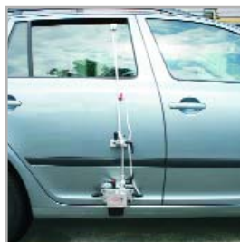
L-350 mounted with a magnetic plate
