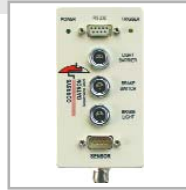
Triggerbox Computer Interface box for CeCalWin and data acquisition via COM port (RS 232)
