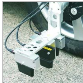
DCA System with SFII-P mounted at the wheel
