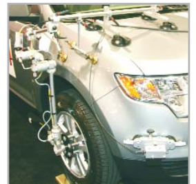
RV-4 Sensor with 4-point suction mount
